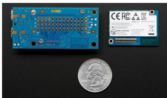
FIG. 25. REGULATOR BREAKOUT BOARD: The above figure shows the size of the regular breakout board on the left, and the size of an Intel Edison microcontroller on the right. [28]
