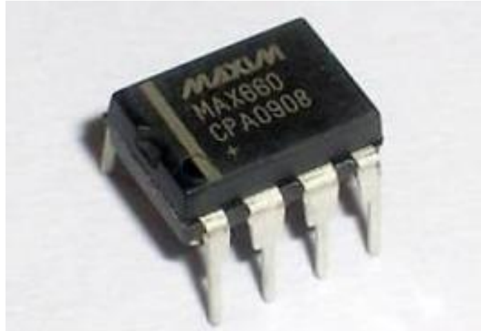
FIG. 32. MAX660 SWITCHED CAPACITOR VOLTAGE CONVERTER:
