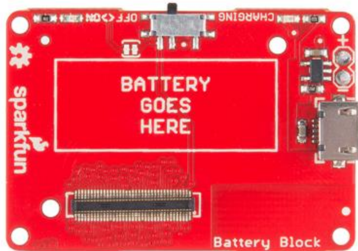
FIG. 30. BATTERY SPARKFUN BLOCK FOR THE INTEL EDISON USED IN THE DEPLOYABLE PROTOTYPE: The deployable prototype uses the battery block to power the intel Edison and the ADC blocks. It is also used as a charger for the battery [36].
