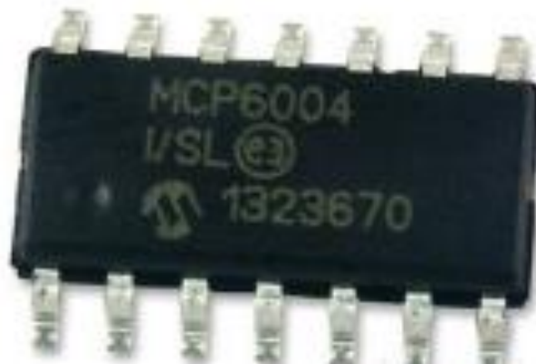
FIG. 31. MCP 6004 OP-AMP USED FOR THE ACQUISITION CIRCUIT: This Op-amp is the chip used for monitoring the resistance change of the sensors [37].
