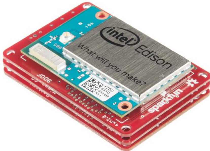
FIG. 28. INTEL EDISON MICROCONTROLLER BEING USED IN DEPLOYABLE PROTOTYPE:
